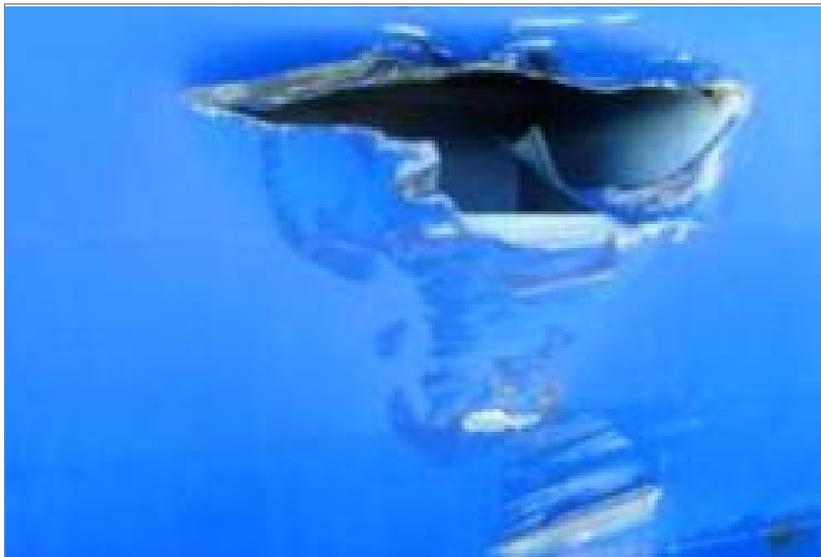
*The tanker's shellplate was breached following an allision with another vessel.*
